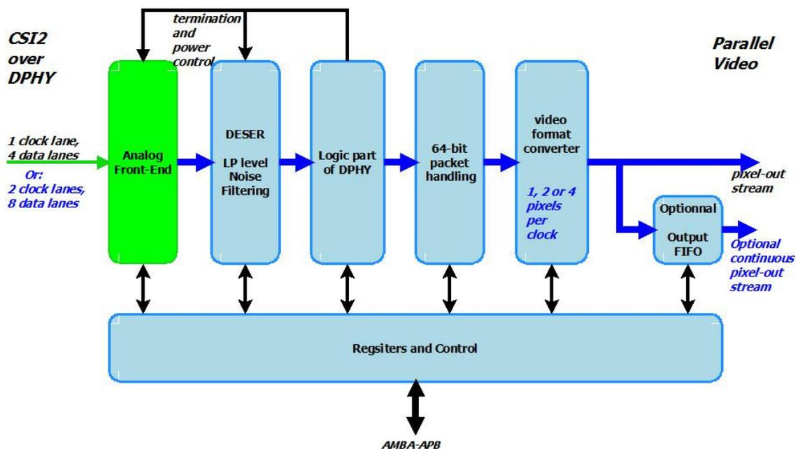
The SVRPlus-CSI2-I-4X can handle from 1 to 4 data lanes. The SVRPlus-CSI2-I-8X , can handle up to 8 data lanes, with one or two clock lanes, and at up to 1.5Gbps per lane.
