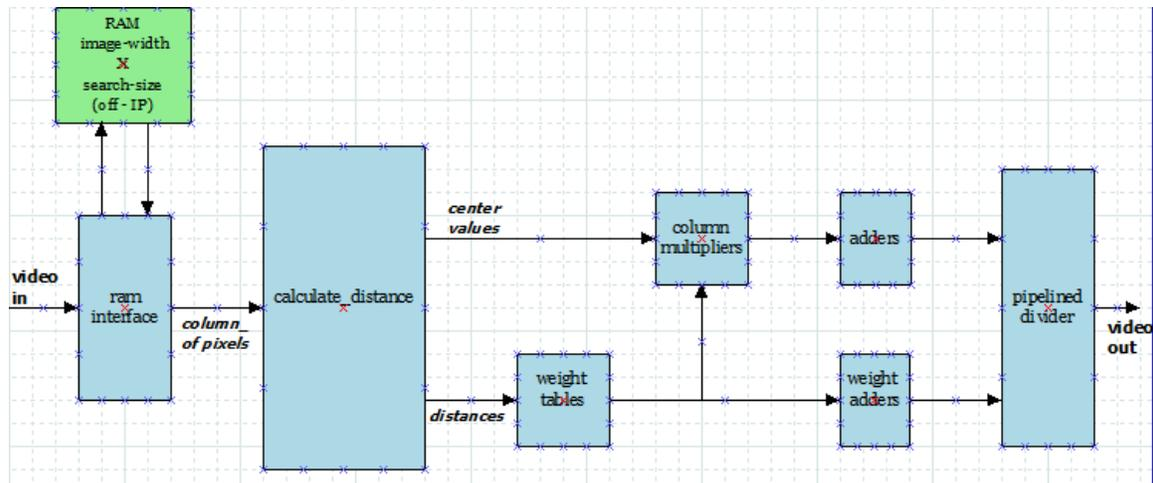
The figure above depicts a simplified block diagram of the V-NLM01 IP. Incoming pixels are handled by a RAM-interface unit, which stores previous rows in an off-IP RAM, and outputs a column of  $N-1$  pixels ( $N$  is the height of the search window).
